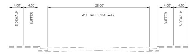
Figure 5: Existing Typical Section Eastridge Drive Looking Northwest
